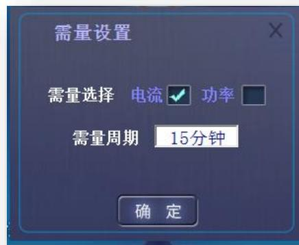
A dialog box titled "需量设置" (Demand Setting) with a close button (X) in the top right corner. It contains two radio buttons for "需量选择" (Demand Selection): "电流" (Current) which is selected, and "功率" (Power) which is not. Below this is a text input field for "需量周期" (Demand Cycle) with the value "15分钟" (15 minutes). At the bottom, there is a "确定" (OK) button.
